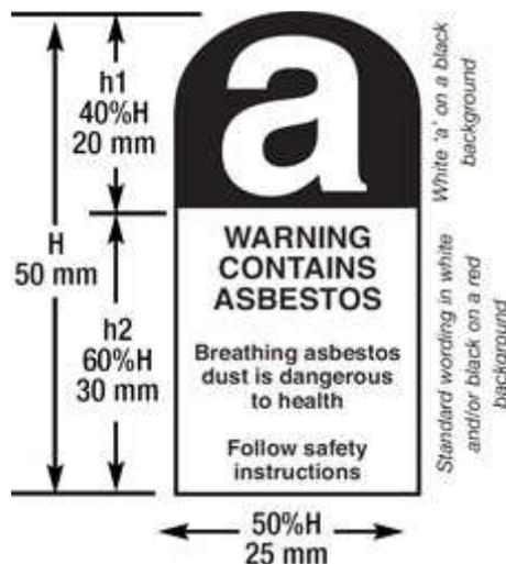
Standard practice is to use a red inner bag, marked up with asbestos warning labels, and a clear outer bag with appropriate hazard markings. Intact asbestos cement sheets and textured coatings that are firmly attached to a board should not be broken up into smaller pieces. These should instead be carefully double wrapped in suitable polythene sheeting (1000 gauge) and labelled.
